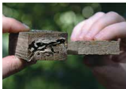
Untreated wood (left), LP SmartSide (right)
